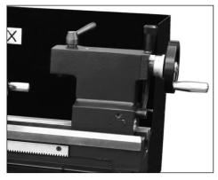
The tailstock may be moved along the bed to any desired position and is secured in position by a quickly locking handle (behind the tailstock and at the right end). The Tailstock spindle carries an internal No.2 Morse taper for use with the Center provided. A Revolving Live Center and Drill Chuck are also available from your dealer. (See Accessories)
