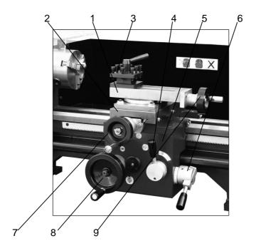
The position of the tool is effected by turning the cross-slide feed handle (7), which moves it across the lathe, and the carriage/saddle or manual feed handle (8), which moves it longitudinally. Additionally the compound slide feed handle (9) may be used to move the tool by small amounts at right angles to the cross-slide. The slide may be set at an angle to the cross-slide so that short tapers or bevels may be cut. This is described in greater detail under 'Bevel Cutting'.
